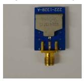
(c) Patch Antenna Working at 4.5 GHzFigure 5: Three Sets of Antenna used in Measurement
